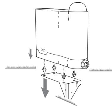
1. Push the mounting bracket into the ground until the top is flush with surface. Use a blunt piece of wood as a mallet, if necessary.
