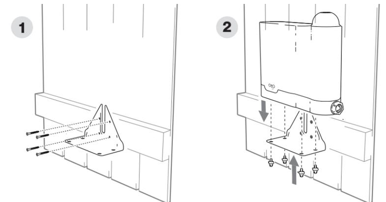
1. Use the four included screws to secure the bracket into a wood fence.
